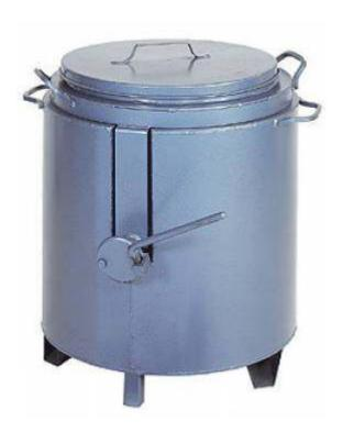
15 Gallon Tar Pot Kit. Manufactured from heavy gauge steel. Welded to highest standards. Removeable inner tank. c/w Heavy Duty Burner, adjustable regulator, 0 - 4 bar and 12 feet of armoured hose. Fitted with adjustable pouring tap.
