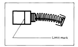
Use a screwdriver to remove the brush holder caps. Take out the worn carbon brushes, insert the new ones and secure the brush holder caps.
