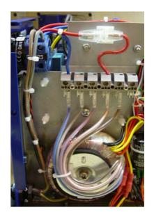
NOTE! Never attach the input tapping wire to the 220V terminal.
