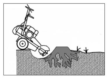
Make sure the throttle is set to "MAX". The cutter wheel is thus accelerated to cutting speed.
